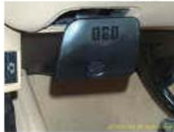
16 Pins (OBDII) DLC under dashboard beside the steering
